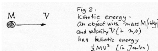
In the same way **wind is kinetic energy**; it has mass and it is moving. How can we make good use of this energy? Let us first try and get an idea of how much energy (or power) there is in the wind.
